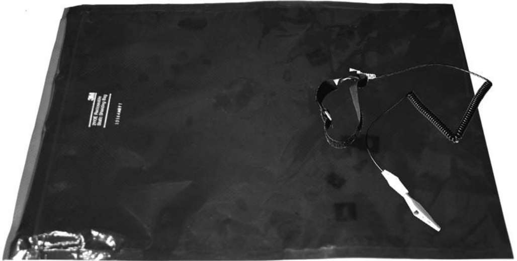
FIGURE A.13 Antistatic protection is necessary both while you are working and when you store parts.
