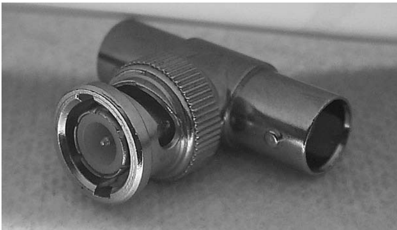
FIGURE B.5 The BNC connector on this T-connector is a form of bayonet connector.
