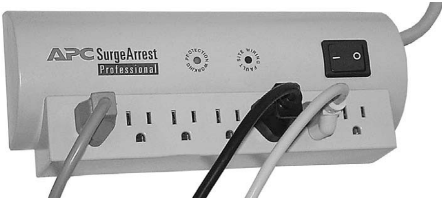
FIGURE S.10 A good surge suppressor should be standard equipment on every computer system.
