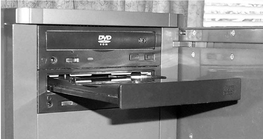
FIGURE T.5 Trays are the most common disk holder used in optical drives.
