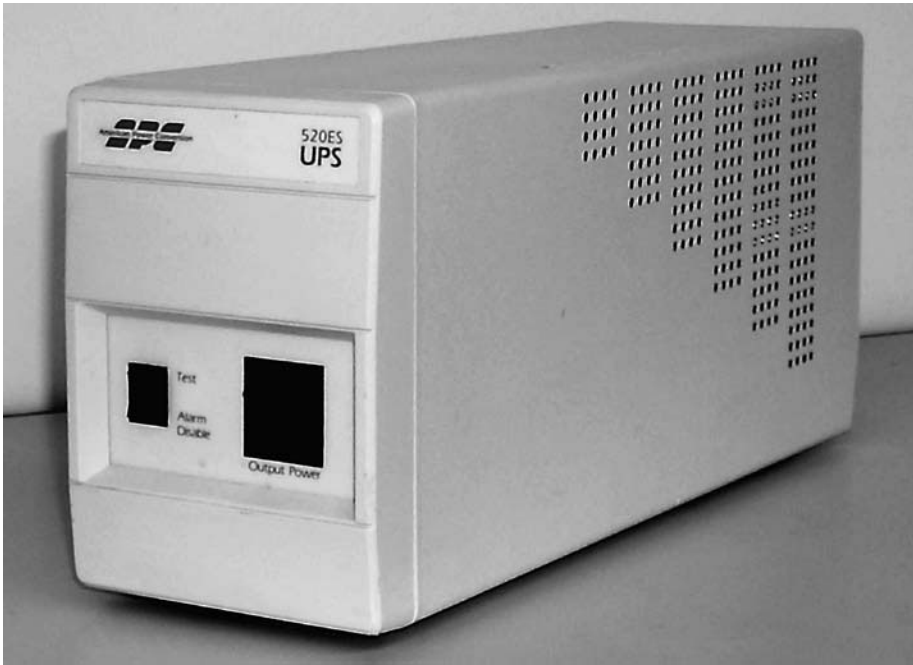
FIGURE U.1 A UPS is a necessary device for any computer system that contains critical data. It prevents a power outage from abruptly shutting down the system.
