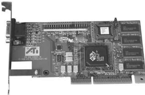
FIGURE A.4 For many years AGP video cards dominated the market. PCI-X and PCI Express have since moved in on their territory.
