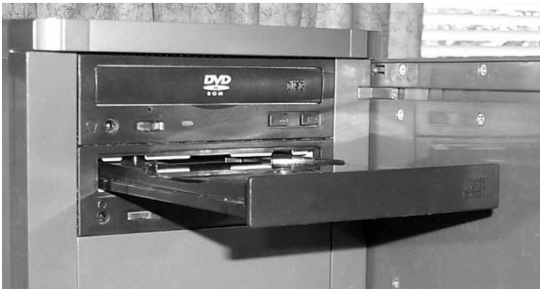
FIGURE B.6 The bezel on this CDR covers the internal mechanisms and provides support for the eject key and a status light.
