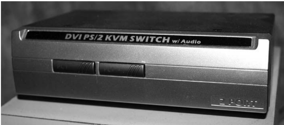
FIGURE K.3 KVM switches range from this inexpensive dual-PC device all the way up to rack-mounted devices that cost thousands of dollars and support many computers.
