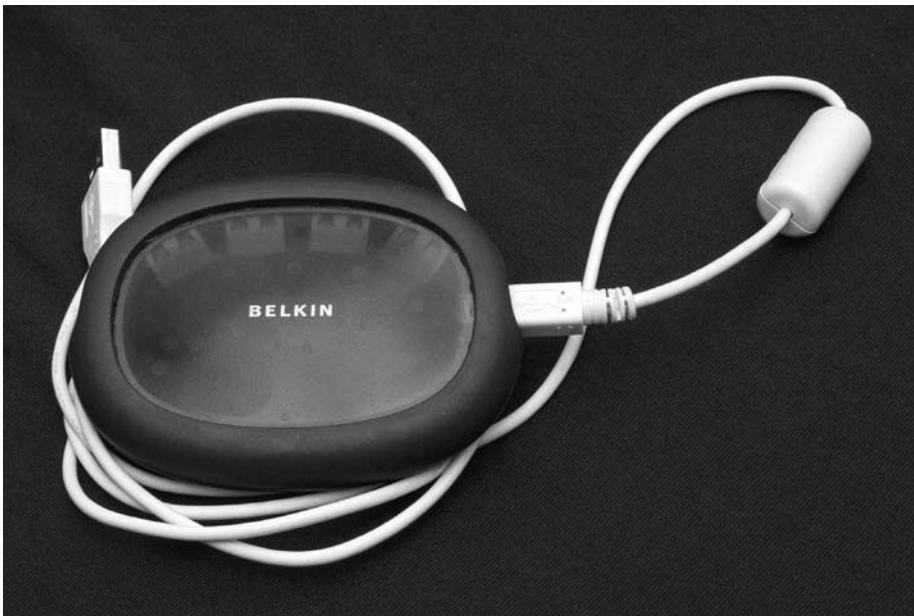
FIGURE U.2 USB hubs are available as simple external devices that let you hook up additional USB devices to your system.
